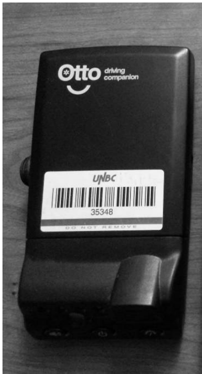
Figure 1. Persentech Otto hitchhiker units modified to gather information on hitchhikers by pressing Group, Couple, Unknown, Female, or Male buttons. A red error button was later added.
